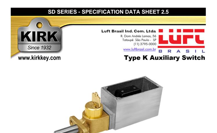
The Type K auxiliary switch is a quick-make, quick-break device capable of handling relatively large currents. The switch is mounted on the end of the interlock as shown. The Type K auxiliary switch can be mounted on the following interlocks:
